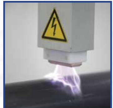
Corona treatment of extruded pipes before printing
