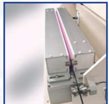
Corona treatment of electrical cable treatment prior to printing
