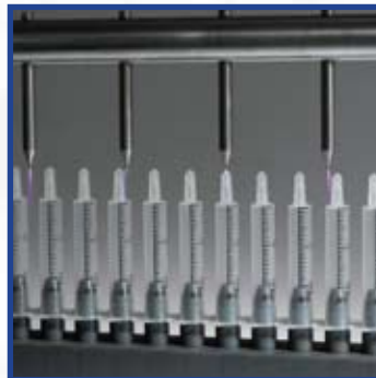
Corona treatment of needle hubs before gluing
